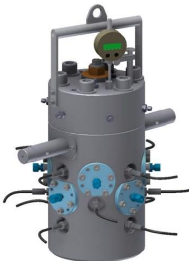
Figure 1. 3D image of the high-pressure acoustic cell
